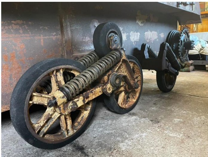
Right: Assembled right hand side centre bogie with both spring sets and return roller fitted.
