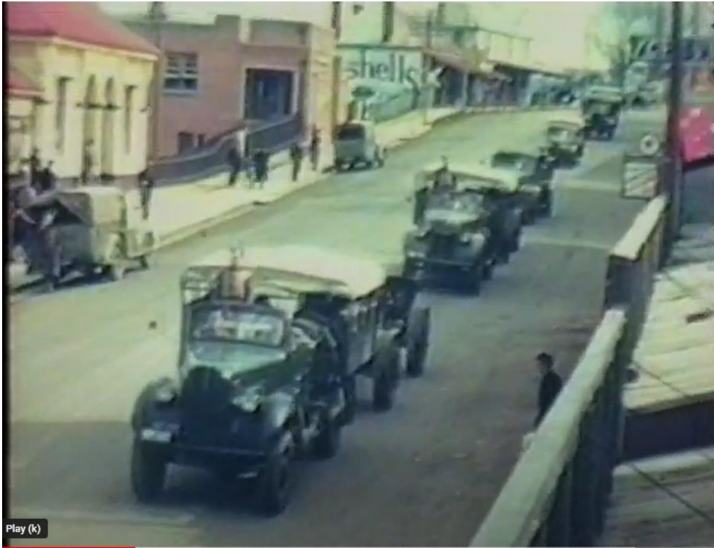
Above: 0min 32 Sec – Another LP3 Gun Tractor also towing a 4.5inch howitzer with limber. This is the same type of Gun Tractor as at 0min 25 sec (with the “beer barrel” type grill). The second Gun Tractor in this image has a different grill and is the later 1940 Ford O1T, possibly making it an LP3A Gun Tractor?
