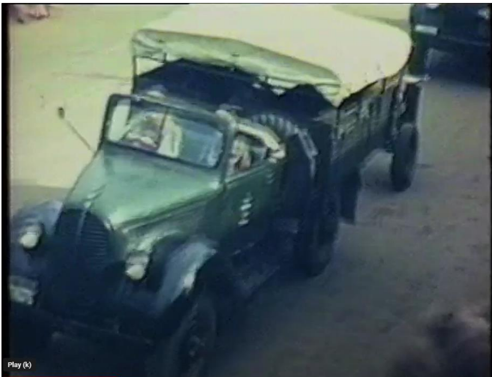
Above: 0min 41sec – Close up of a Ford LP3 Gun Tractor with the “beer barrel” type grill. This one is towing a 2Pdr Anti-tank gun. This shot shows some good features of the LP3 Gun Tractor, with driven Marmon Herrington Front axle and “Roadster” cab.
