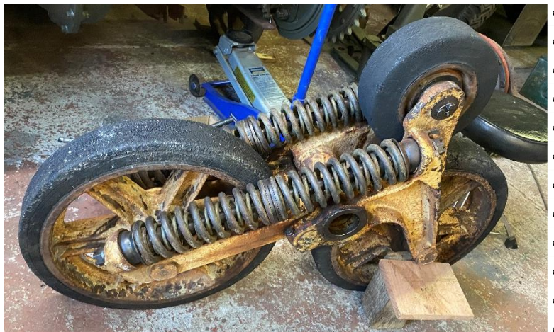
Left: Left hand side centre and rear bogie on Carrier 2814 with refurbished suspension.
