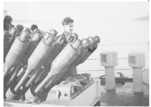
The Hedgehog anti-submarine weapon on board HMAS Murchison in the Han estuary, Korea 1951
