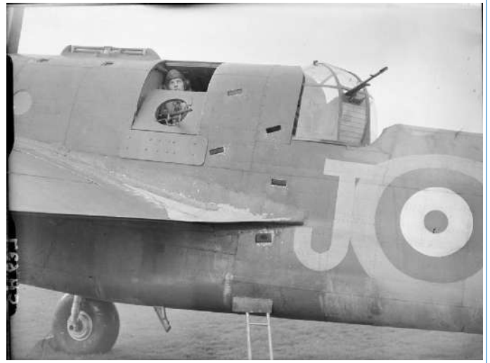
Beaufort L4461 'OA-J', of No. 22 Squadron RAF. The turret has a Vickers K machine gun; for protection against beam attacks, another K gun is mounted in the port entry hatch.
