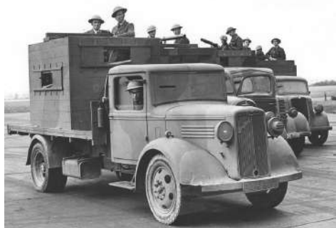
Improvised armour added to a truck by railway shop workers for the Danish resistance movement near the end of World War II
