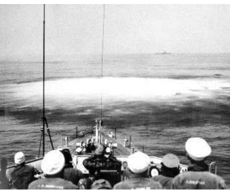
A large white upwelling of water from an underwater explosion just ahead of Moberly's bow following Hedgehog launch
