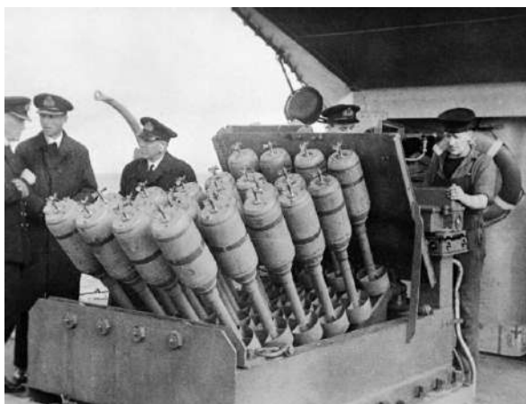
Anti-Submarine Weapons: Hedgehog, a 24 barrelled anti-submarine mortar mounted on the forecastle of HMS Westcott.
