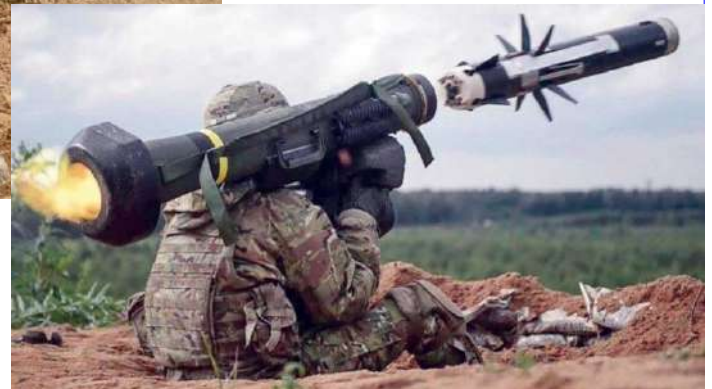
The Javelin Close Combat Missile System – Medium (CCMS-M) is a man-portable, medium-range tactical missile system that provides the U.S. Army and Marine Corps with precision direct-fire effects to defeat main battle tanks and other armored vehicles.
