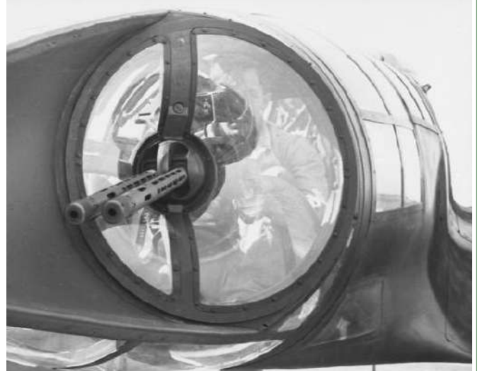
The rotatable, Ikaria-designed twin barrel machine gun mounting in the crew nacelle's tail cone
